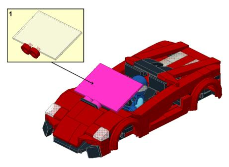
To connect the Windshield 4X5 use two Anetenna Base (4592) instead of two round plates w/ shaft 3.2 (20482)
